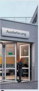
Folding doors made of steel and aluminium
