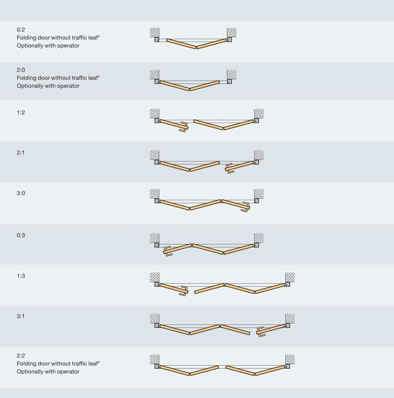
Folding arrangements are read from left to right on the opening side. Further folding arrangements on request. (see also the technical manual).
